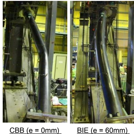
Deformation shape in compression (1.5% story drift)
