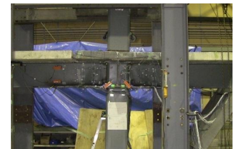
Test of the repaired connection
